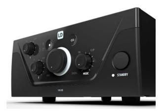
The LD Systems IMA installation mixer amplifier is suitable for low impedance or 70V/100V line loudspeaker circuits. A Hi-Z / Lo-Z selector switch enables complete separation of the output signal from the output transformer to ensure an optimal frequency response for low impedance applications.
