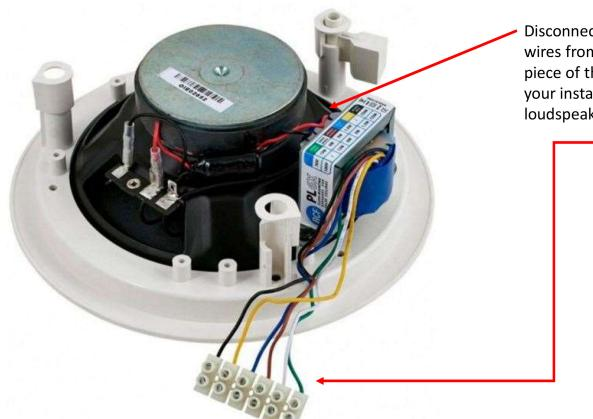
Disconnect / Cut the Red and Black wires from the transformer and using a piece of the connector strip connect your installed cables directly to the loudspeaker.
