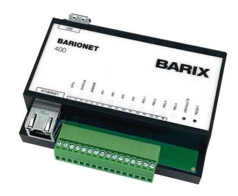
Barionet 400 is a fully programmable I/O device server of Barix, based on Linux/Lede/OpenWRT. The device features most common IO interfaces such as USB, digital Inputs and Relays. It is IPv4 or IPv6 capable. Supporting multiple communication protocols, the Barionet device can be used in different applications such as automation, building control, public transport and many more. Barix Products are developed in Switzerland and manufactured to the highest standards.
