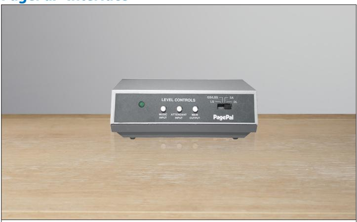
The PagePal® unit interfaces with most phone systems to virtually any public address audio system. In addition, PagePal furnishes inputs for background music and auxiliary inputs for microphones, radio receivers and recorded announcements. Control inputs are provided for tones generated by PagePal. This device is not recommended for talkback.
