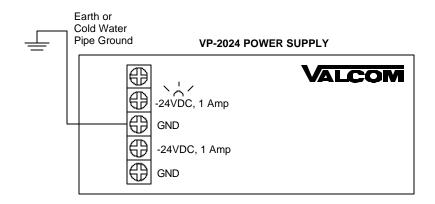
Figure 1 - Power Connections to Valcom Page Control Units
