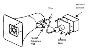
Figure 3 - Mounting to an Electrical Backbox
