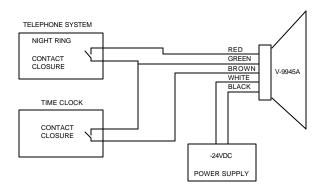
FIGURE 1 - TYPICAL INSTALLATION
