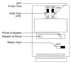
Location of Screw Terminals, Option Switches and Volume Controls
