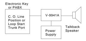
Figure 1 - Typical Loop Start Trunk Installation
