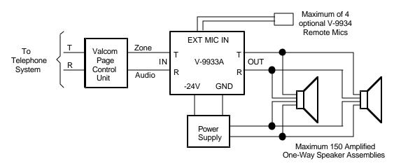
Figure 2 - Simplified Block Diagram of Connections
