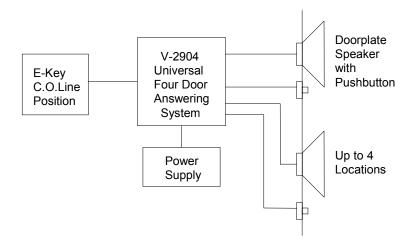
FIGURE 1 - SIMPLIFIED BLOCK DIAGRAM OF A TYPICAL INSTALLATION
