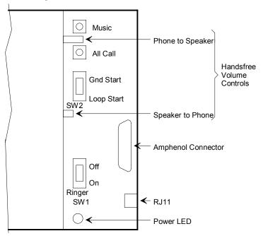
Figure 3 - Connector and Control Locations
