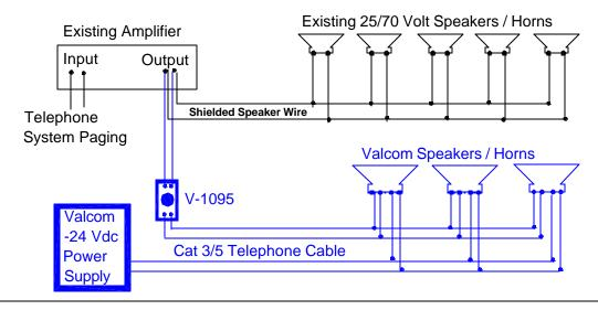
In situations where it is not practical to run a new wire from the amplifier location to the new speakers/horns location, use the V-1095, 25/70-Volt Expand to tap into an existing 25/70-Volt speaker wire run.
