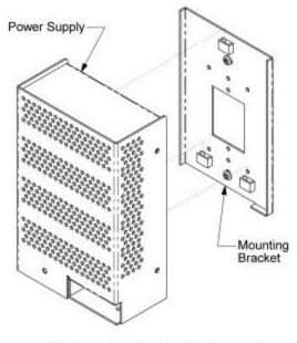
Figure 4. Mounting the Power Supply
