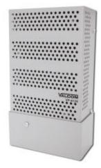
with respect to ground. The regulator will maintain 24 Volts +/- 2% over the rated range of input voltages and output loads. A greater than 4 Amp load on power up will cause the power supply to current limit. Short circuit protection is provided. Overvoltage is provided to limit the output voltage to approximately 28 Volts should a failure occur within the power supply. Outputs may be used in a series for 48V @ 2A.
