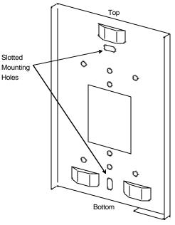
Figure 3. Mounting Bracket
