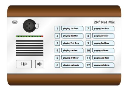
Initial View of 2N® Net Mic via 2N® IP Audio Control Panel
