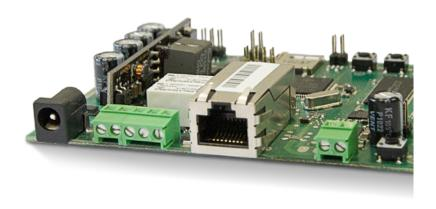
2N® Net Audio Decoder mono PCB, Part No. 914050E
